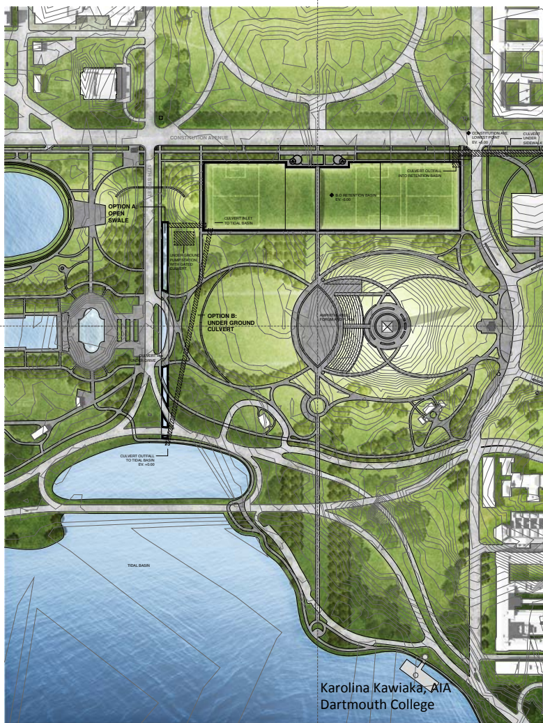
MONUMENT GROUNDS - RETENTION AREA WHEN EMPTY - SWALE OR CULVERT TO TIDAL BASIN
